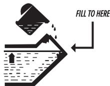
**Recommended motor oil:** SAE 10W30, SAE 10W40.
